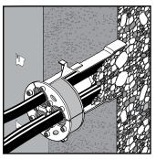
The seal can also be installed from the inside of the structure.
