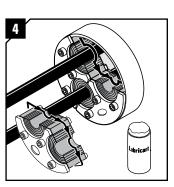
Lubricate the inside surfaces all around with Roxtec Lubricant, especially into the corners. Continue reinstallation from step 7.
