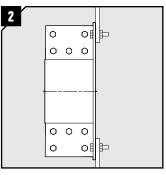
Use the flange as template for the drilling of the bolt holes.
