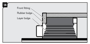
Sectional view of the seal showing when rubber expands and bulges. The required torque depends on several things, e.g cable or pipe size, amount of used lubricant, sleeve size or material in the cable sheath.
