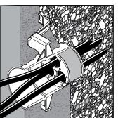
The seal can be installed from the outside of the structure.
