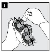
Lubricate the three parts of the seal all around.
