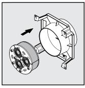
The seal must always be installed in the correct end of the knock out sleeve.
