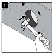
Remove the knock-out of the sleeve before inserting the seal.
