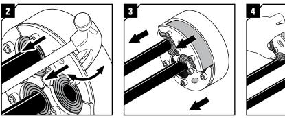
Use a suitable tool to remove the halves of the H3 seal. Be careful not to damage the seal.
