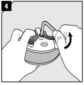
Make sure that the bolts of the seal are loose.
