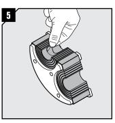
Adapt rubber layers to fit the cables.
