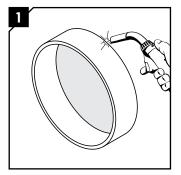
Weld the Roxtec sleeve to the cabinet/wall. Welding guidelines are available at www.roxtec.com.
