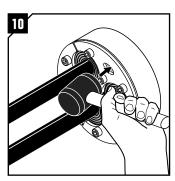
If necessary, use a rubber hammer.
