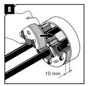
Insert the seal into the sleeve. Leave a 10 mm margin to simplify the installation of the last piece.
