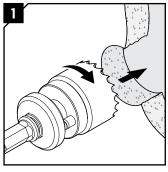
Installation of seal into a core-drilled hole. Use a hole saw with the appropriate diameter.
