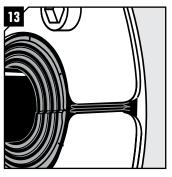
The seal is compressed when the rubber expands through the fittings and when the inner part bulges.
