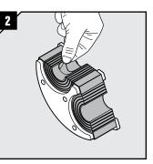
Adapt halves, which are to hold the additional cables or pipes, by peeling off layers until you reach the gap seen in pic. 3. The number of layers may not differ by more than one between the halves.
