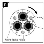
Tighten the screws crosswise one turn at a time. Start with the inner screws.
