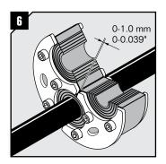
Test with a cable. Achieve a gap of 0-1.0 mm between the rubber halves. Adapt the layers for all cables. The halves may not differ by more than one layer.
