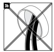
Pull the pipes/cables through. Cables shall go straight through the seal.
