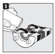
Lubricate thoroughly on the inside and sparsely on the outside of the rubber surfaces of the seal with Roxtec Lubricant. No need to apply lubricant to the grey intumescent material.
