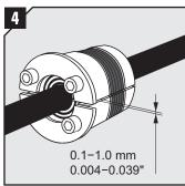
Try to achieve a 0.1-1.0 mm gap between the two halves when held against the pipe.
