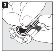
Adapt the seal to the pipe by peeling off layers from the halves until you reach the gap seen in pic.4. The halves may not differ by more than one layer.
