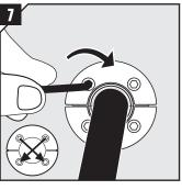
Tighten the screws crosswise. This will compress and seal the RS PPS/S. See table for approx. torque. See fig. 1 and 2 for reference.
